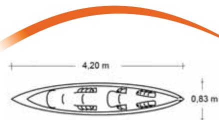
WEIGHT 34 kg - MATERIAL: POLYETHYLENE
