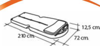
WEIGHT 14 kg - MATERIAL: POLYETHYLENE
