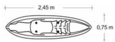
WEIGHT 23 kg - MATERIAL: POLYETHYLENE
