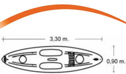
WEIGHT 22 kg - MATERIAL: POLYETHYLENE
